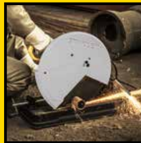
9 Cutting Rebars, Steel Beams, Angle Iron Chop Saw STEL701
